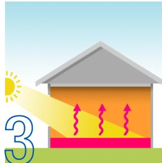
Thermal Mass (concrete, masonry, structurally insulated panel construction)
