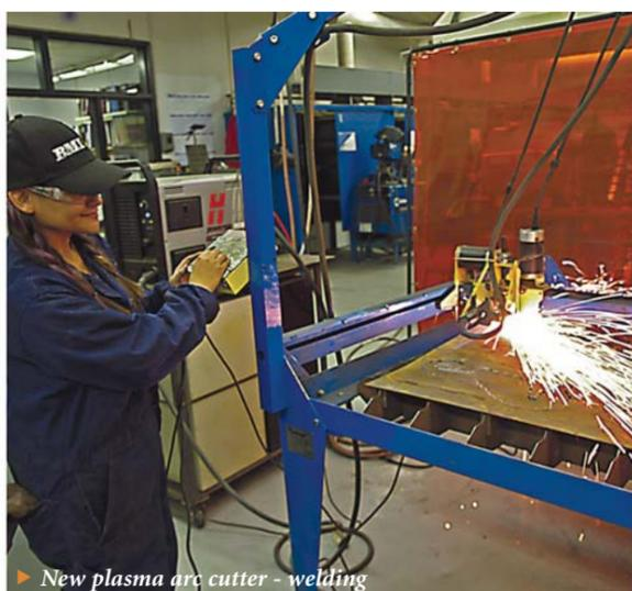
▶ New plasma arc cutter - welding
