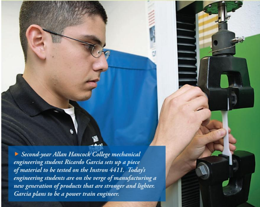
▶ Second-year Allan Hancock College mechanical engineering student Ricardo Garcia sets up a piece of material to be tested on the Instron 4411. Today's engineering students are on the verge of manufacturing a new generation of products that are stronger and lighter. Garcia plans to be a power train engineer.
