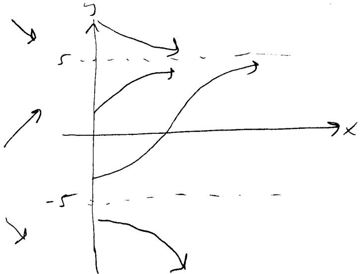
$$y'' = -2y \cdot y' \quad \begin{array}{l} \text{if } y > 5, y'' \text{ is } + \\ \text{if } -5 < y < 5, y'' \text{ is } + \\ \text{if } 0 < y < 5, y'' \text{ is } - \end{array}$$
