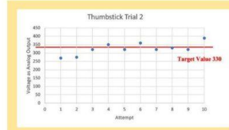
Figure 2. Shows values of attempt of trial 2 using the thumbstick to grab a water bottle. 50% of the time the flex sensor performed on target or \pm 10 units of the target value while still maintaining a grip without squishing it. The other attempts ranged from \pm 20 to \pm 60 .
