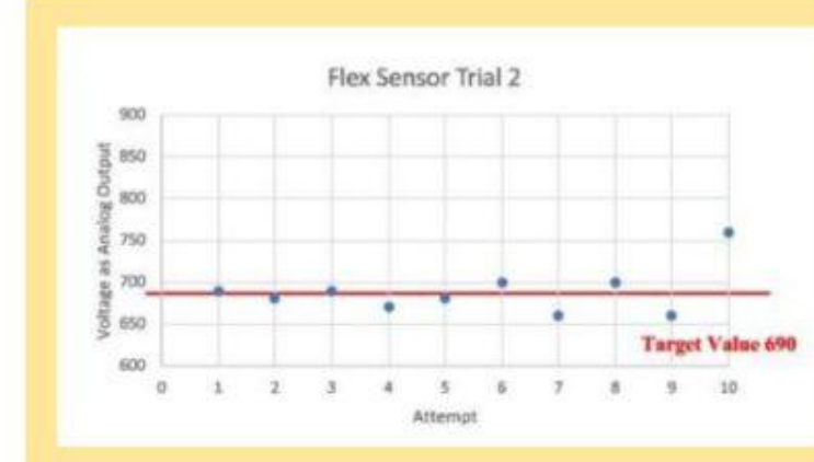
Figure 4. Shows values of each attempt of trial 2 using the flex sensor to grab a water bottle. 60% of the time the flex sensor performed on target or \pm 10 units of the target value while maintaining a grip without squashing the bottle. The other attempts were close by about \pm 20 except for one outlier.
