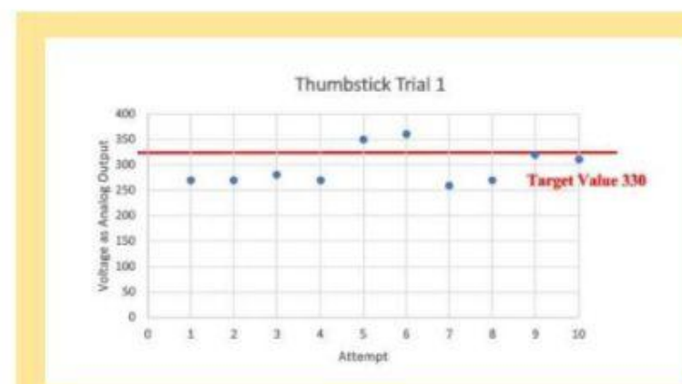
Figure 1. Shows values of attempt of trial 1 using the thumbstick to grab a water bottle. 20% of the time the flex sensor performed on target or \pm 10 units of the target value while still maintaining a grip without squishing it. The other attempts ranged from \pm 20 to \pm 70 .
